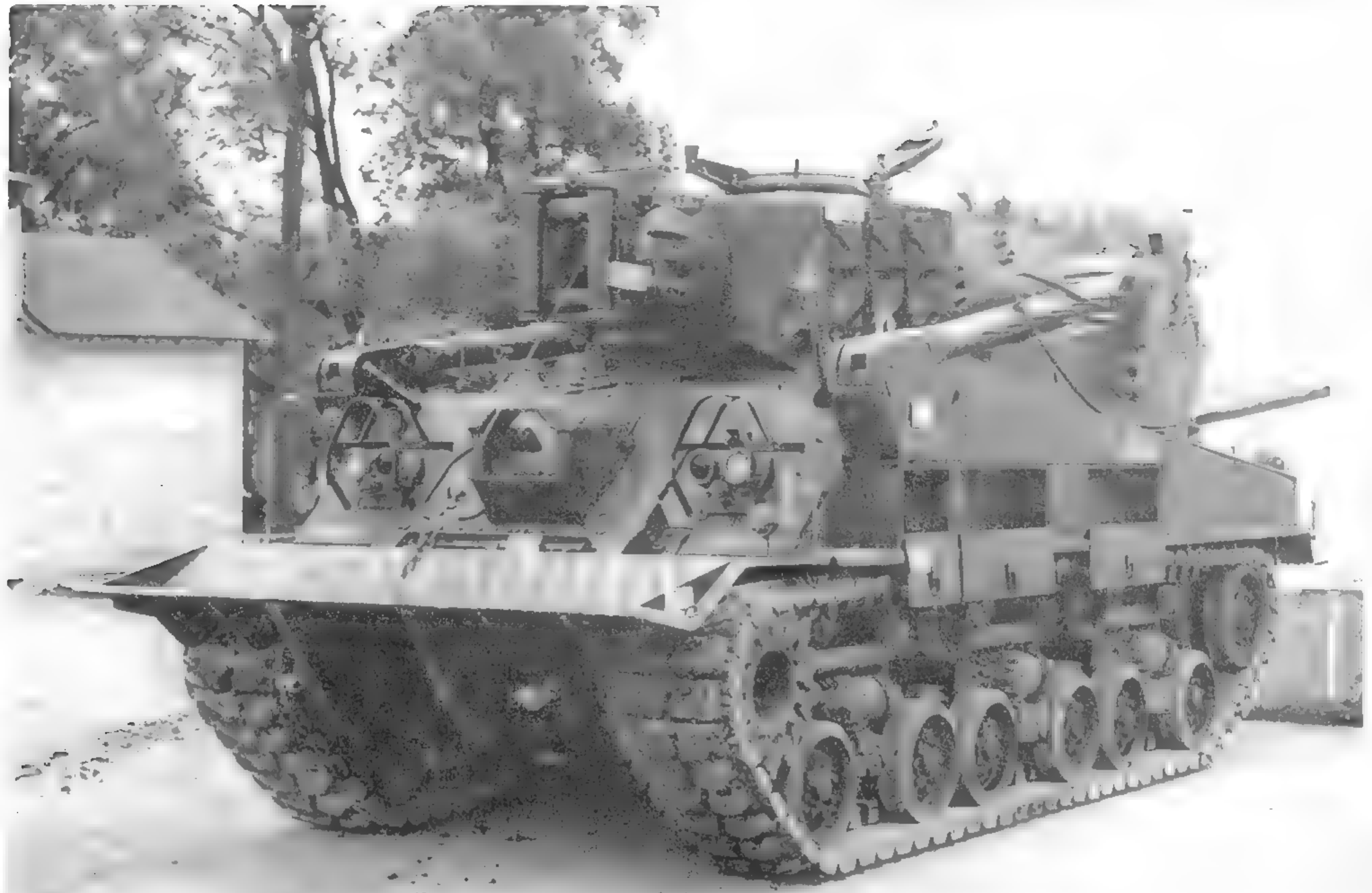
The M74 blade was raised by attaching the rope from either the auxiliary winch (mounted on "turret" face), or the main recovery winch, whose rope played out of the opening in the glacis plate. The stowage compartments mounted along the sides of the vehicle were a welcome improvement over the stowage arrangement of the M32 series vehicles. (Photo courtesy of the Patton Museum)
